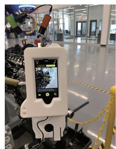
IBM Maximo Visual Inspection app at client site, inspecting engines
